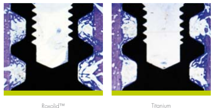
Fig. 2: Histological analysis showing Roxolid™ (left) and titanium (right). They have shown a better bone in-growth behavior of Roxolid™ compared to pure titanium 4
